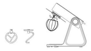
8. The bowl is fixed/removed from the host by turning in the lock/unlock direction as below.
